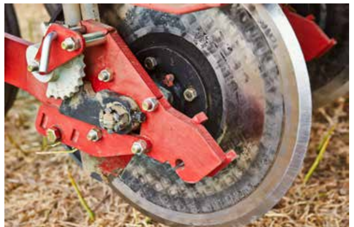
Walking beam design for better penetration ability at higher speeds
